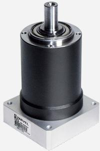
The reduced backlash planetary speed reducers, Series RG, are designed as one and two stage versions, with hardened and tempered steel housing and broached internal gear.
